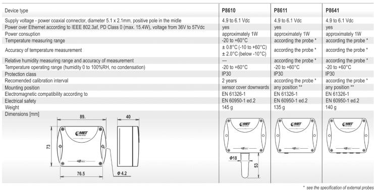
\*\* the device with attached DSRH/C or DST/C probe install always vertically with the sensor cover downwards
