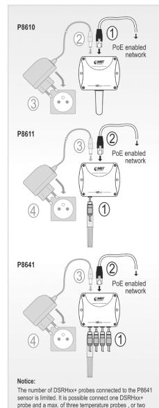
DSRHxx+ probes and a max. of one temperature probe.
