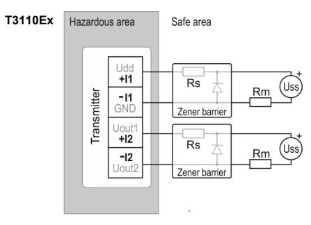
Loop resistance value Rc = Rm + Rs + resistance of wiresshall fulfill the condition  $Rc[\Omega] < 40 \times Uss[V] - 360$ .
