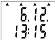
If battery voltage drop occurred since last internal clock setting below critical limit or battery disconnection for longer period than approximately 30 s, after display switch ON (during date and time display) all four arrows appears as warning to check or set it again from the computer. However all logger functions work without limitation.
