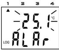
Active alarm is indicated (if display is ON) by blinking of the value on the display and reading ALAR appears at the LCD lower line at the same time. **Notice:** if logger is operated at low temperature (below approximately -5 °C), alarm indication by blinking can be indistinct. Indication by the ALAR reading works correctly. If alarm is active reading MIN/MAX is disabled (if selected).
