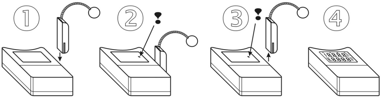
**Switching the logger OFF by magnet**
