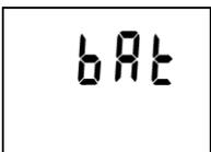
If reading BAT is displayed permanently, battery voltage is low and logger is not possible to switch ON. If logger was switched ON before it, data logging is stopped and logger is switched OFF. Communication with computer can temporarily work. Replace battery as soon as possible!
