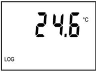
**If display is switched ON**, actual reading of measured values is displayed - channel 1 temperature (°C 1) on the LCD upper line, channel 2 temperature (°C 2) on the LCD lower line. Symbol LOG indicates data logging in progress – if it blinks, data memory is filled up to more than 90%.
