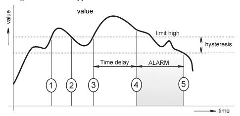
In Point 1 the measured value exceeded the limit. From this time, the time-delay is counting. Because at point 2 the value dropped below the limit value before the time delay expired, alarm was not set.
