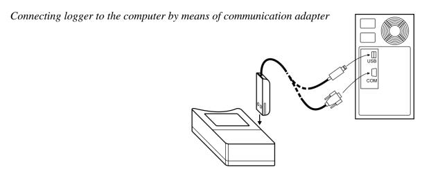
Notice: USB connector can be located also from the computer front side
